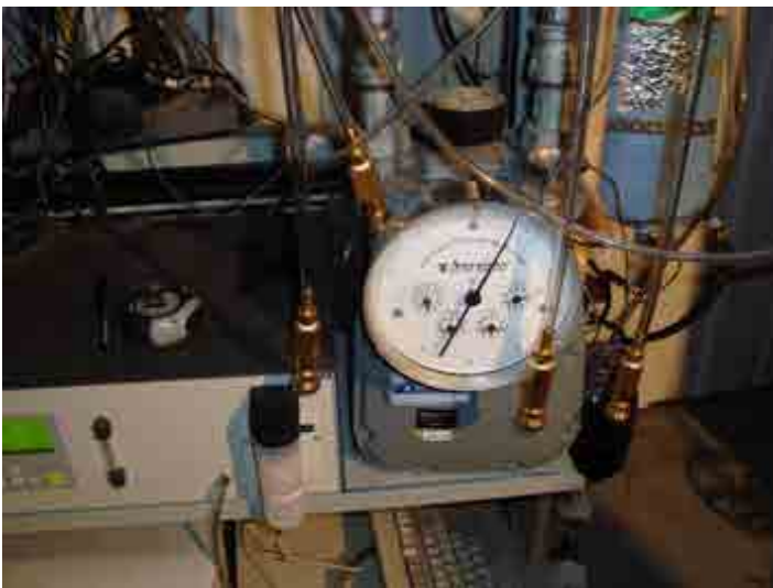
Picture 8: Reference dry gas meter
